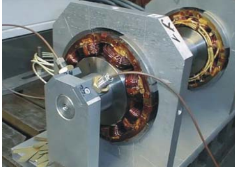
Figure 1. Magnetic bearing demonstrator with two radial bearings (max. force 230 N)
