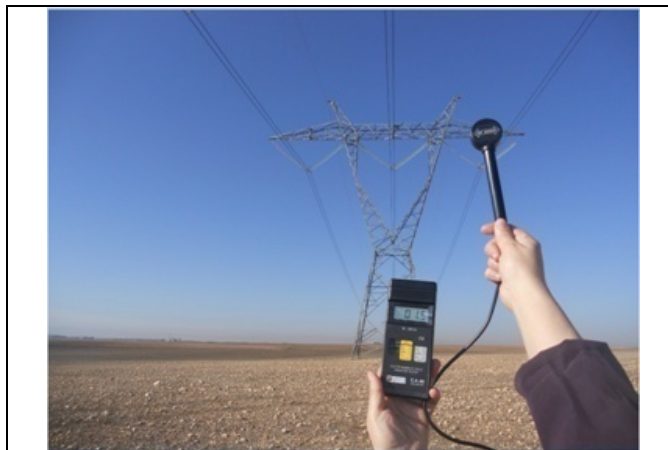
Fig.11.magnetic induction measurement for 400kV line
