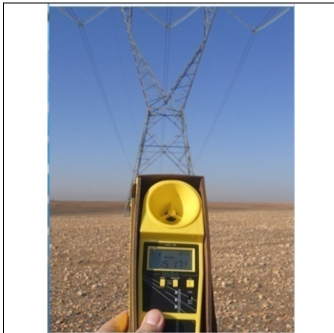
Fig.12. Height measurement between ground and conductor
