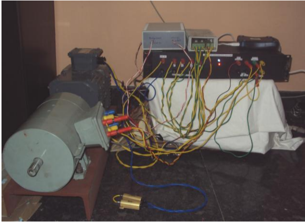
Fig. 5. Practical set-up of DC Shunt Motor under Test
