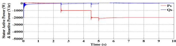
Fig. 9. Stator active power and reactive power during variable speed operation
