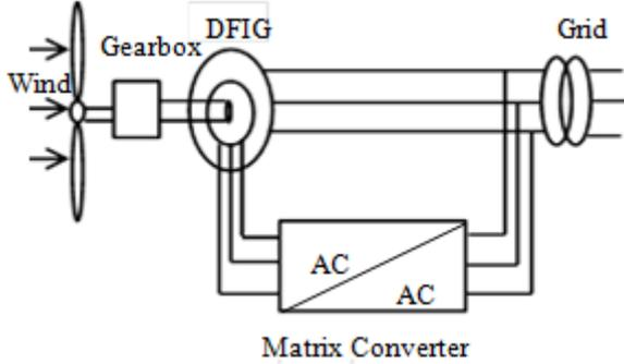
Fig.2. DFIG – WT with the MC
