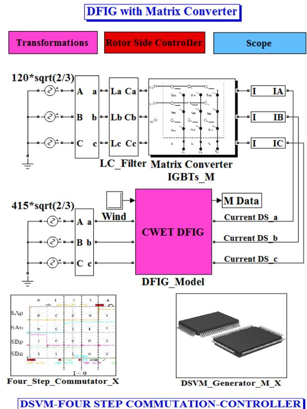
Fig.5. Matlab/Simulink implementation of the proposed control of the DFIG-WT connected to the MC
