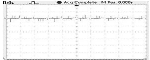
Fig.19. Stator active power at super-synchronous speed
