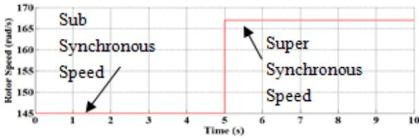
Fig. 6. Variable speed operation of the rotor
