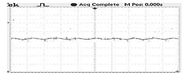
Fig.20. Stator reactive power at super-synchronous speed
