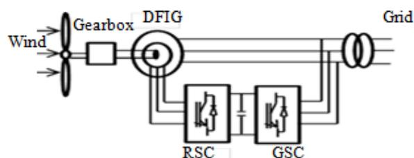
Fig.1. DFIG-WT with the Back to Back Converter
