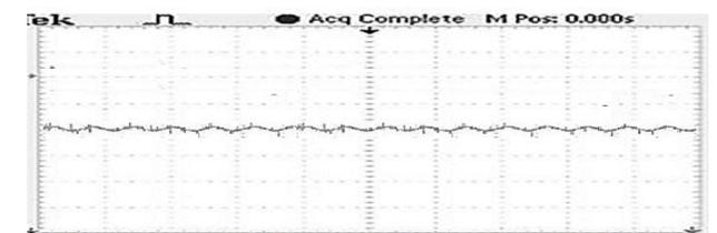
Fig.22. Stator reactive power at sub-synchronous speed
