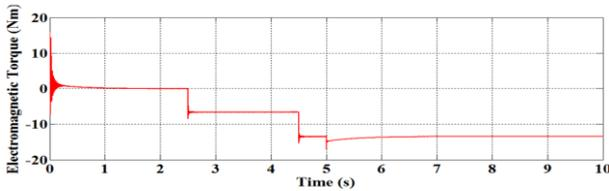
Fig.8. Electromagnetic torque during variable speed
