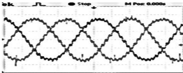
Fig.17. Output currents of the MC
