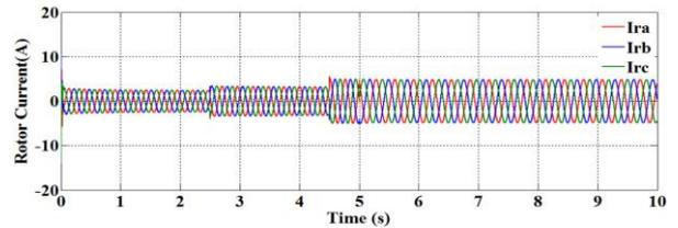
Fig. 12. Rotor current under variable speed operation
