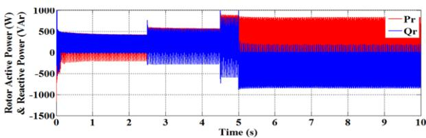
Fig. 10. Rotor active power and reactive power during variable speed operation
