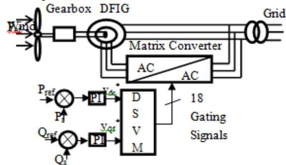
Fig.4. Block diagram of the proposed control of DFIG -WT connected to the MC
