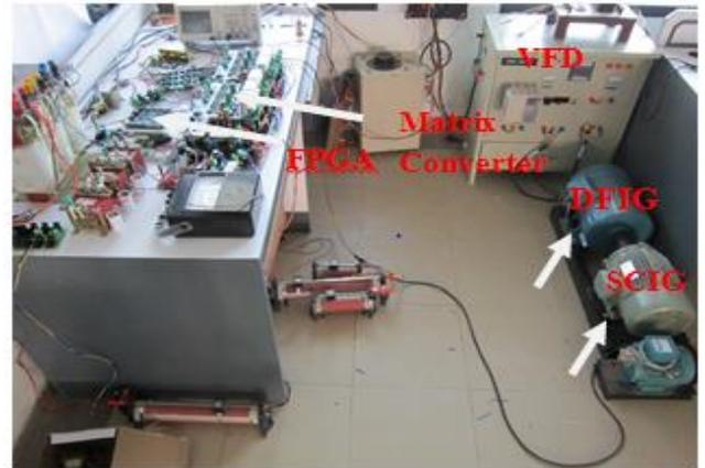
Fig. 14 Laboratory setup for the stator power control of the DFIG-WT connected to the MC at the rotor using FPGA-SPARTAN 3E Controller
