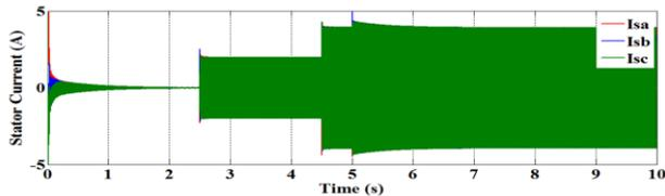
Fig. 7. Stator current during the variable speed operation
