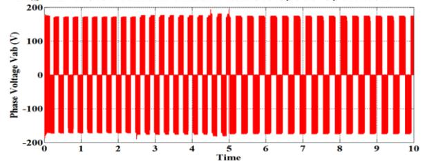
Fig. 13. Rotor phase voltage  $V_{ab}$  under variable speed
