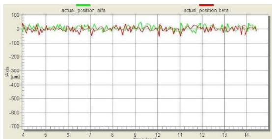
Fig. 4-2 Levitation of the rotor around centre of the stator bore
