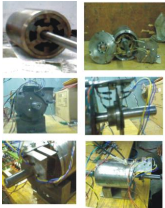
Fig.14. The entire assembly process displaying the windings on the stator, slotted disk fixed to shaft, fixing photo sensors for position sensing and the associated wiring.
