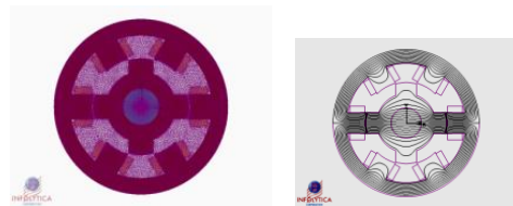
Fig. 4. Finite element mesh and the Flux lines plot for SMC1000-SRM.
