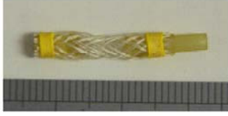
Figure 3: Components of ECF micro artificial muscle actuator
