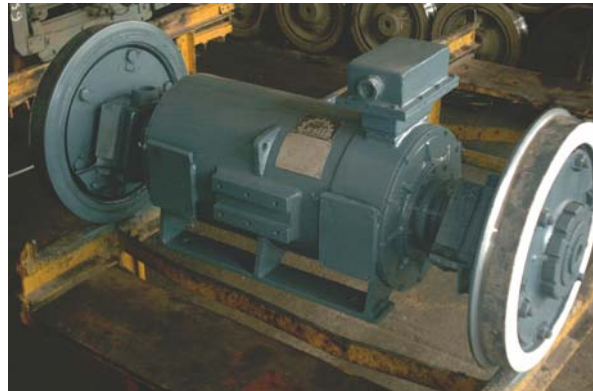
Figure 3. The wheel-set with motor prototype.
