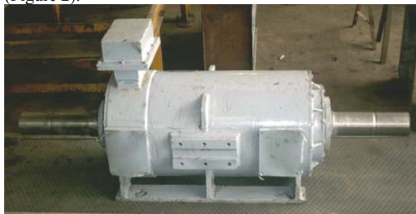
Figure 2. The motor prototype and actual wheel-axle.
