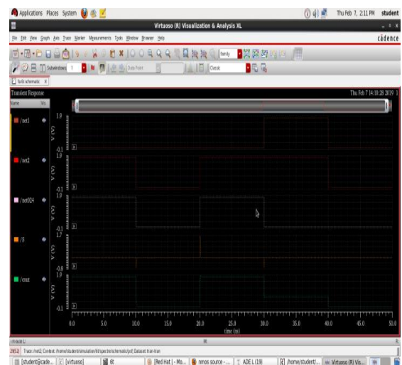
Fig. 2. 2 Simulation output of Full Adder
