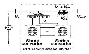
The basic function of convertor1 is to supply or absorb the real power demanded by convertor2 at the common DC link to support the real power exchange resulting from the series voltage injection. This DC link power demand of convertor2 is converted back to AC by convertor1 and coupled to the transmission line bus via a shunt connected transformer.
