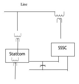
The reactive power exchanged at the AC terminal is generated internally by the convertor. The real power exchanged at the AC terminal is converted into DC power which appears at the DC link as a positive or negative real power demand.
