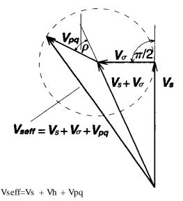
The phase angle diagram has been shown above using Hybrid model of the UPFC controller.
