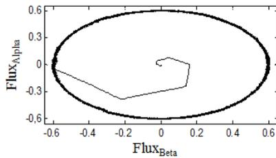
Fig. 13. Zoom on the stator flux waveform.
