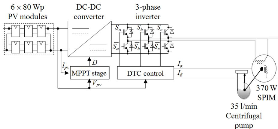
Fig. 1. General architecture of the photovoltaic-powered pumping application.
