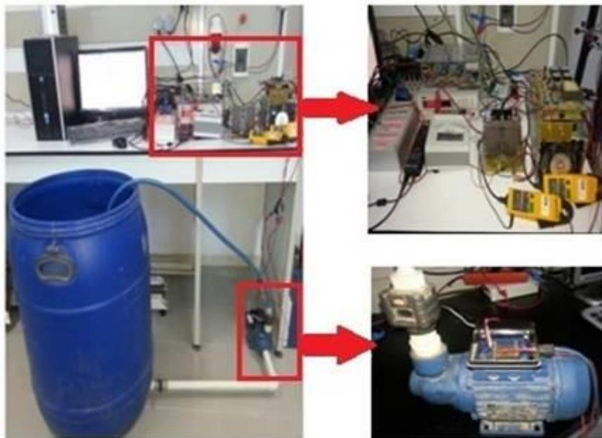
Fig. 16. Experimental test bench of the PV-pumping system.
