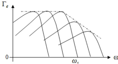
Fig. 5. Torque-speed curve.
