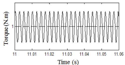
Fig. 11. Zoom on the electromagnetic torque waveform.
