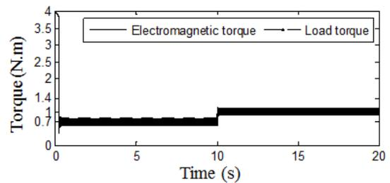
Fig. 10. Electromagnetic torque waveform.
