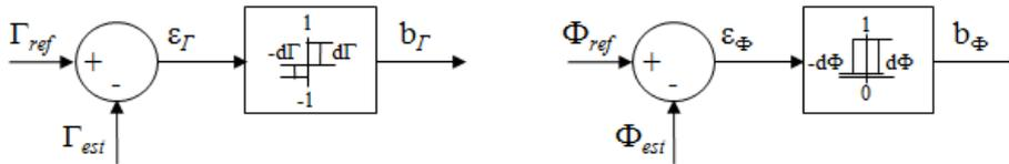
Fig. 8. General outline schematic of 3-level hysteresis regulator.
