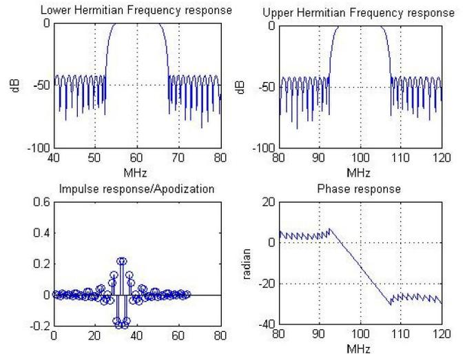
**Figure 6:** effect of the change in maximum passband ripples from 0.5db to 1db at the same substrate and same other parameters of figures 3, and 4.
