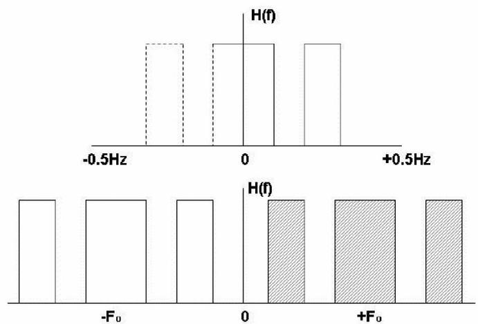
**Figure 2:** Baseband response (upper) and bandpass response (lower) of a 3-passband SAW filter.
