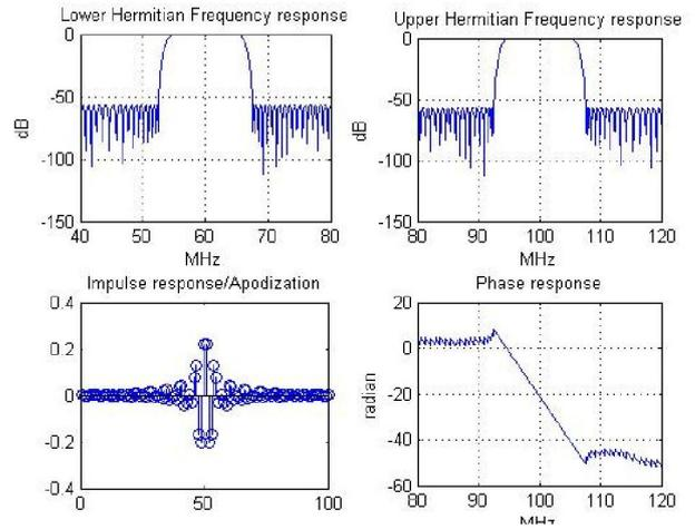
**Figure 5:** affect of changing number of fingers for YZ LiNbO3 substrate from 64 to 100 with the same other previous parameters.
