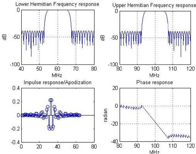
**Figure 4:** different responses of an apodized SAW filter of YZ LiNbO3 substrate, no. of fingers=64, 0.5db passband ripples, and min. stopband=30db.
