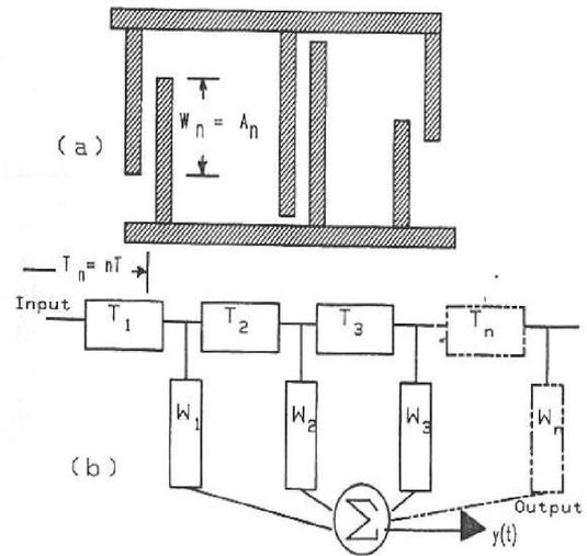
**Figure 1:** (a) Apodized transducer, and (b) delta function – model representation.
