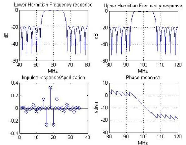
**Figure 7:** effect of the change of minimum stopband attenuation value, when attenuation changed from 30db to 20db.
