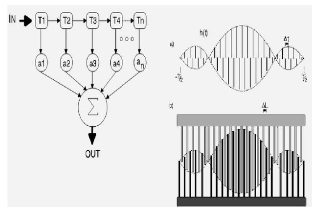
**Figure 3:** Schematic of a Finite Impulse Response (FIR) Filter.
