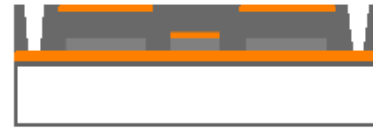
Fig. 13. Etching of sacrificial layer to form anchors.
