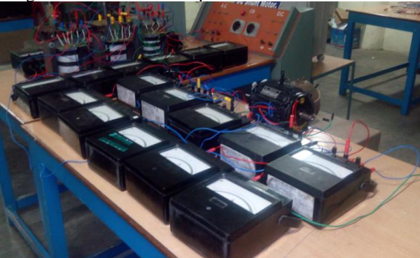
Fig.10. Experimental Setup of Five Phase induction motor drive
