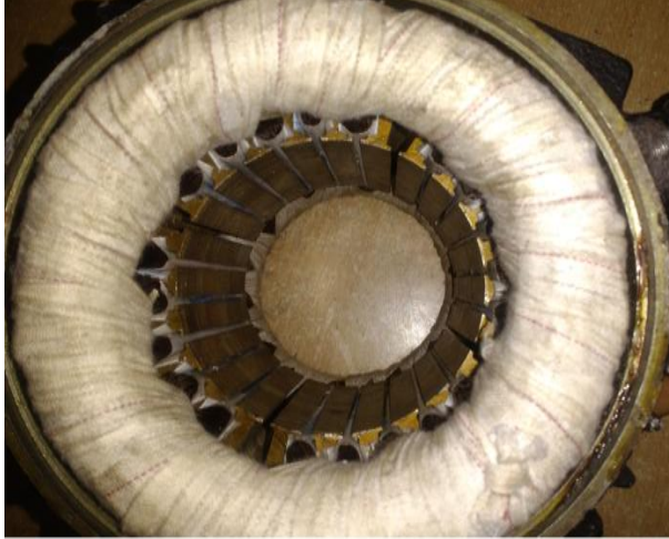
Fig8.Slots with copper windings of five phase induction drive
