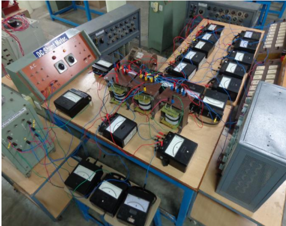
Fig .6.Experimental Setup of Fabricated Five Phase Transformer under Rated Load Testing.
