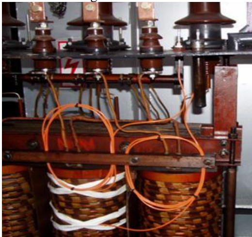
Fig. 4. Position of the optical detectors covered by white stripe
