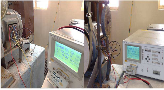
Fig. 4. Experimental setup for DM and CM test of a 5hp induction motor.
