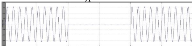
Fig. 6f distorted voltage waveform due to PQ event type3
