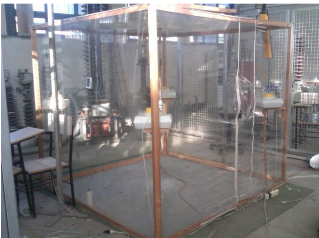
Fig. 3. Fog chamber for experimental tests
