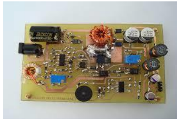
Fig. 7. Prototype implementation of ASM controller
