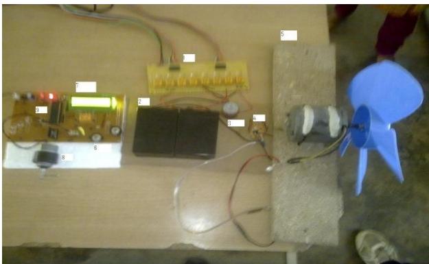
Fig.13 Battery/ super capacitor charging using Wind energy
