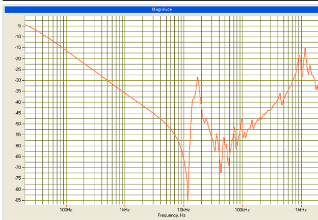
Fig 7. Measurement is taken between high voltage winding and neutral with tertiary short circuited
